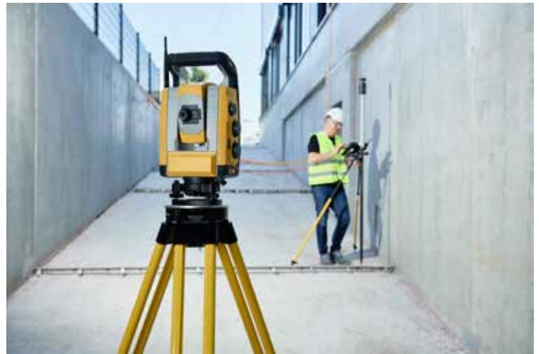
Robotic total stations have dramatically improved construction layout. structural components already in place. In a worst-case scenario, layout errors that are not identified or properly prioritized during construction weaken or otherwise compromise the finished structure, creating a serious safety hazard for occupants.
